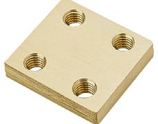
The Short D Plate (Part # 80329001) is made of brass and fastened to the back of a single cylinder SD Series Type D interlock to allow front mounting (see SD Series Data Sheet 1.4). The thickness of the Short D plate is 3/8". To order this plate with your SD Series Type D interlock, put the letter "P" in column fourteen of the interlock part number - reference the SD Series Ordering Guide.
