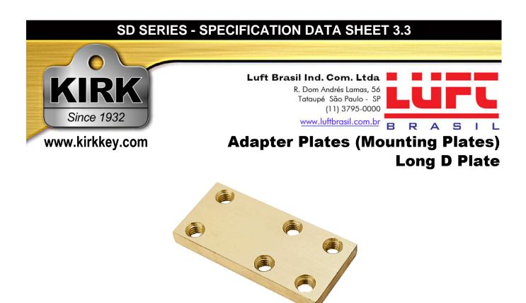
The Long D Plate (Part # 80329002) is made of brass and fastened to the back of a multicylinder SD Series Type D interlock to allow front mounting (see SD Series Data Sheet 1.4). The thickness of the Long D Plate is 3/8". To order this plate with your multi-cylinder SD Series Type D interlock, put the letter "P" in column fourteen of the interlock part number reference the SD Series Ordering Guide.
